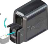
Peel off the center strips on both sides of the adhesive cleaning card.
